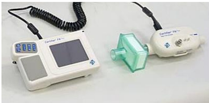
Figure 10. Connecting the Interface Module to a Flow Module
