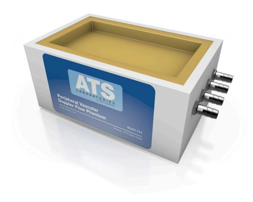
The Models 524 and 525 tissue mimicking Doppler flow phantoms contain four flow channels simulating superficial vasculature. The simulated vessels are located 15 mm below the scan surface. Built-in scanning wells are provided to permit the use of water or a low viscosity gel as acoustic coupling agents.
