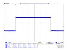
600 µs Pulse Width, 3500 V Output, at load
